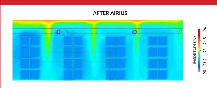
This Airius installation allowed the warehouse to pass FDA Validation Testing and helps ensure the safety of the products for the manufacturer and the consumer. It has been reported to Airius that the temperature variance from the bottom of the 18' racks to the top with the fans running over the last year is only 1 to 2°C.
