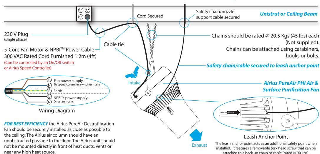
attached to a back up chain or cable (rated @ 90 kgs).
