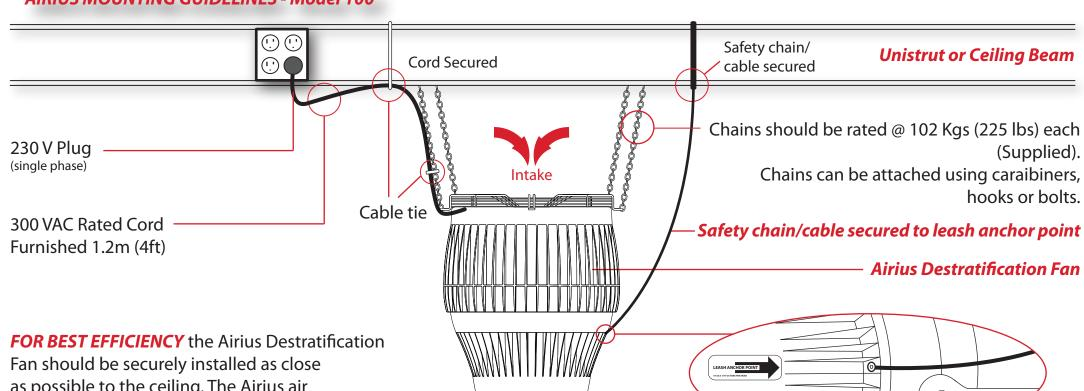
Fan should be securely installed as close as possible to the ceiling. The Airius air column should have an unobstructed passage to the floor. The Airius unit should not be mounted directly in front of heat ducts, vents or near any high heat source.
